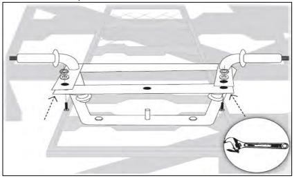
**STEP 5**Position the Central Front Axle Brace (10) up to the Front Axle Support (9).
