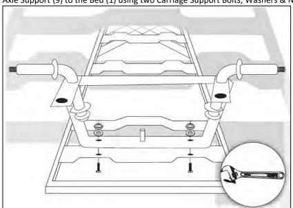
**STEP 4**Attach the Steering Link Connector (12) to the Front Axle Support (9), using Bolts, Washers and Nuts (19). The connector should sit over the axle as pictured.
