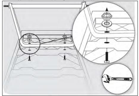
Place the Right (7) and Left (8) Rear Axle Braces onto the Rear Axle Support (6).
