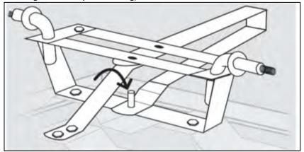
Position the straight arm of the Yoke (11) between the Centre Front Axle Brace (10) & Front Axle Support (9).
