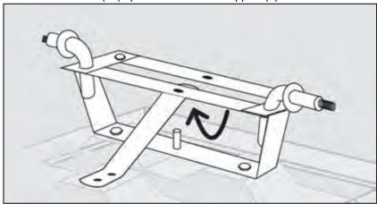
Fix the Central Front Axle Brace (10) to the Bed (1) using Carriage Bolt, Washer & Nut (18).
