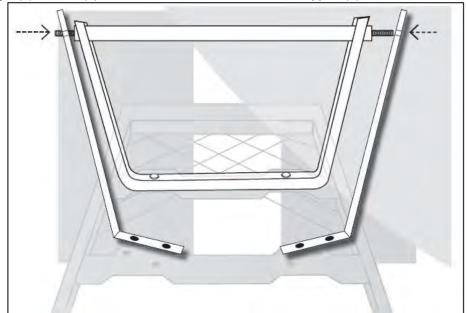
Attach the Rear Axle Braces (7 & 8) to the Bed (1) using four Carriage Support Bolts, Washers & Nuts (18).
