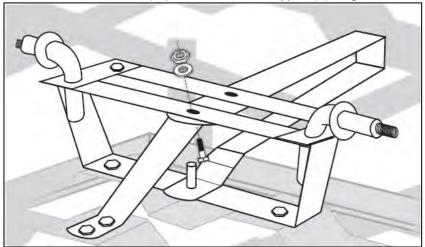
Attach the Steering Link Connector (12) to the Yoke (11) using Carriage Bolt, Washer & Nut (18).
