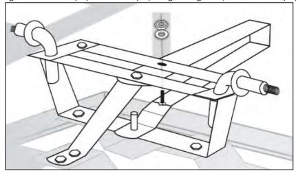
Slide the Large Washer (23) over the Front Axle Support (9) protruding leg (this is stepped) and slide the Split Pin (16) through the hole. Split open the Pin legs to secure.
