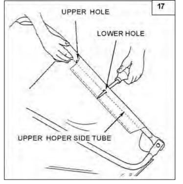
Insert a Ø8X59.5 clevis pin through the lower hole in each upper hopper side tube. Next assemble a bag arm tube onto each clevis pin and secure it with a hair cotter pin Ø3.
