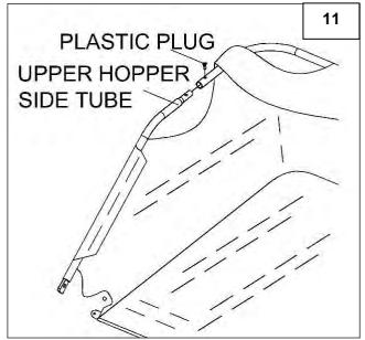
Turn the second rear hopper tube so that the brace holes in the middle of the tube face up. Attach the ends of the rear hopper tube onto the ends of the lower hopper side tubes. Fasten together using plastic plugs.
