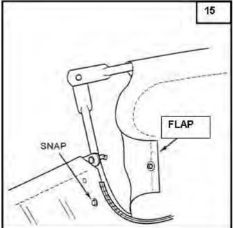
**IMPORTANT:** Do not over bend the support rods during the following step. Over bending will cause the steel rods to lose supporting tension.
